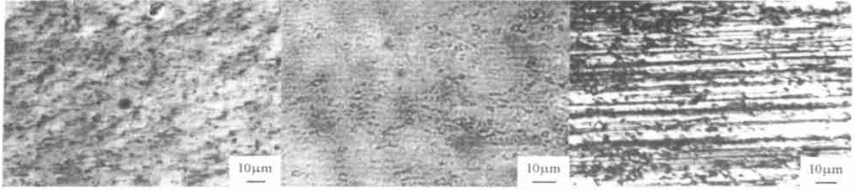
(a) Ni2P 镀层 (98N) (b) Ni2P2纳米金刚石镀层(147N) (c) Ni2P2微米金刚石镀层(196N)
